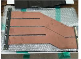
"Flex" cables then connect PCB connectors to ASAD boards High-density cables → capacitance and crosstalk carefully calculated Plugged into "dummy" MM board - no noticeable waveform degradation
